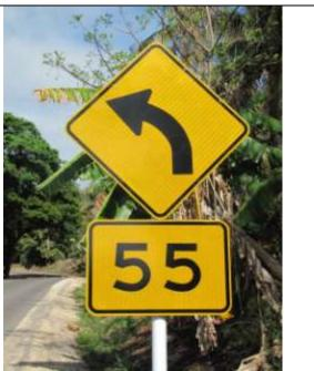
Advisory Speed Sign – this is the safe speed to drive around a corner comfortably. The arrow indicates the direction of the bend and the number is the maximum safe travel speed (in km/hr) for the corner.
